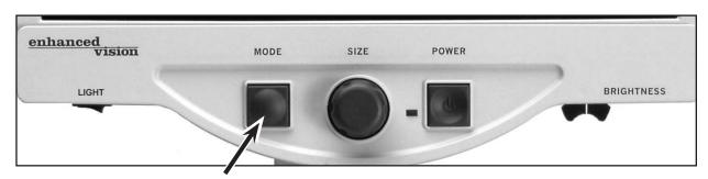
You can choose a viewing option by pressing the MODE button on the control panel. Each press will cycle through all 7 viewing options.
