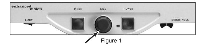
You can increase or decrease the size (magnification) of the image by using the SIZE dial at the center of the control panel (see Figure 1).
