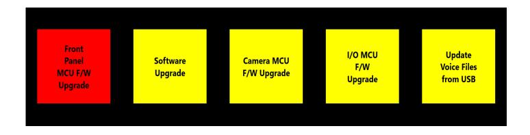
Step 6: For the 01.02.183 Update we need to perform 5 updates for the Front Panel, Software Application, Camera Firmware, I/O Board and Voices which will require you to perform 5 updates in the suggested order Software, Camera, Front Panel, I/O and Voices (Repeat Steps 3-5 for both Software/Voices Upgrade and Camera FW Upgrades). A restart of the system occurs immediately after each component is upgraded and should not be interrupted while in process.
