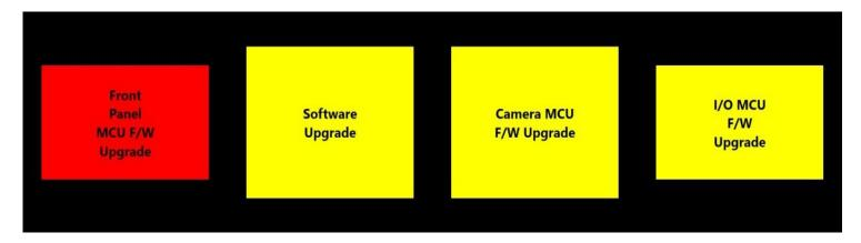
Step 6: For the 01.01.238 Update we need to perform four updates for the Front Panel, Software Application, Camera Firmware and I/O which will require you to perform the update four times (Repeat Steps 3-5 for all Software and Firmware Upgrades). It is recommended that you update the Software First and then the rest. A restart of the system occurs immediately after each component is upgraded and should not be interrupted while in process.
