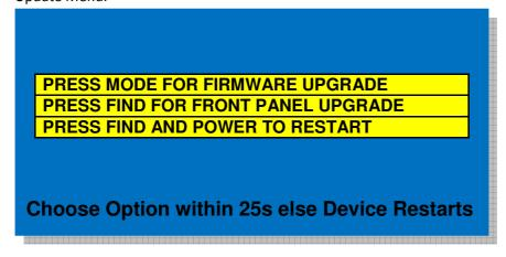
3.) Pres the MODE button to enter firmware update mode in preparation for updating the Main Board Firmware.
