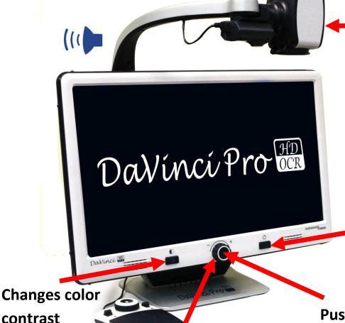
Swivel camera head to change viewing target
